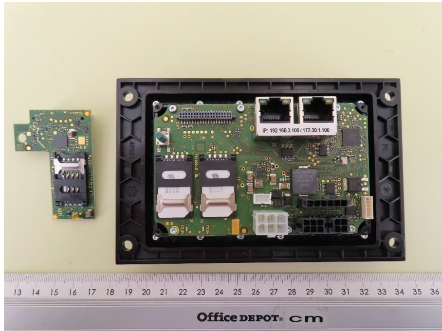
EUT, PCB PAY cVEND EXT-LTE-A removed
