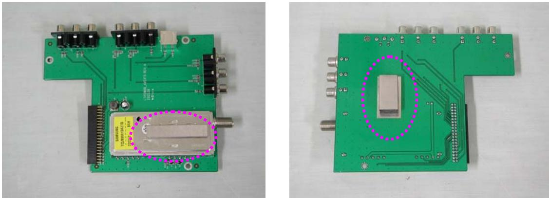
5. Attach a gasket on the main board.
