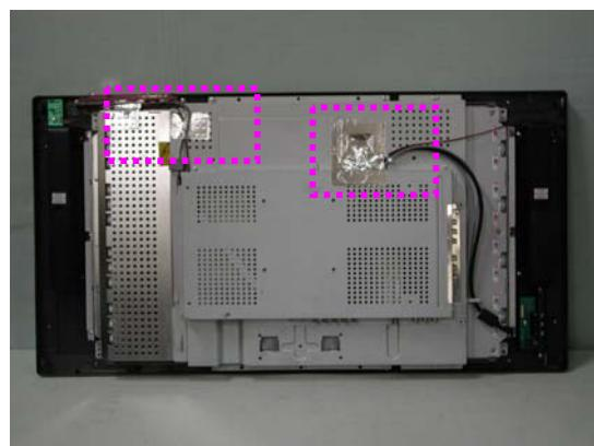
2. Attach a gasket on the main frame cover inside.
