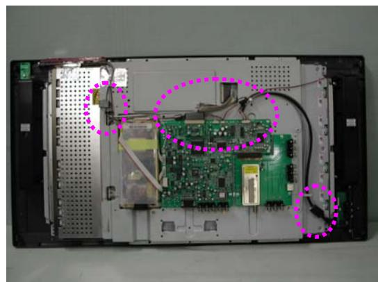
4. Attach a gasket on the tuner and tuner board.
