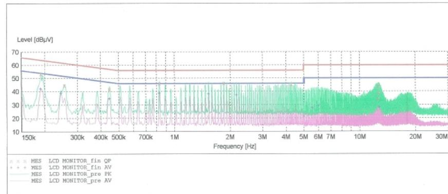
**MEASUREMENT RESULT: "LCD MONITOR\_fin QP"**
