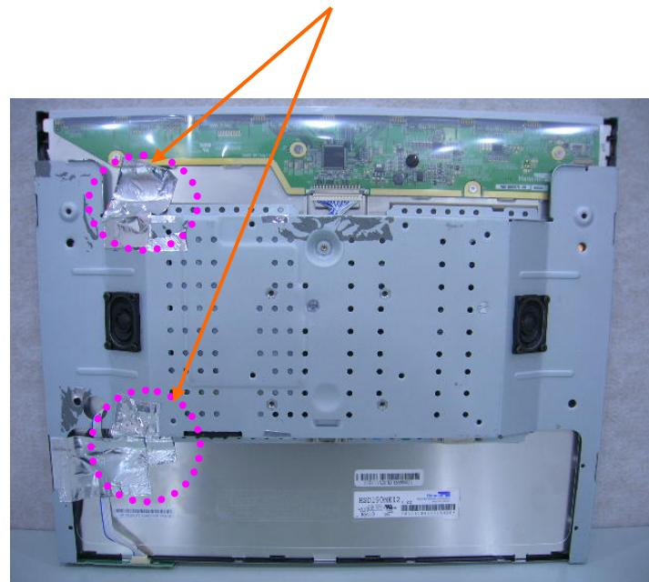
**2. Attach a gasket on the main frame and main board to contact the LCD Rear panel**
