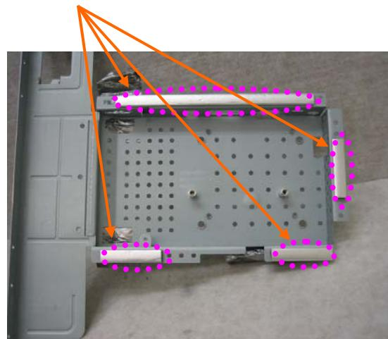
**2. Attach a gasket on the main board to contact the main frame**
