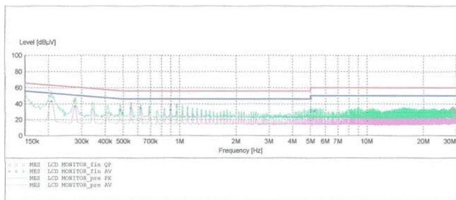
**MEASUREMENT RESULT: "LCD MONITOR\_fin QP"**
