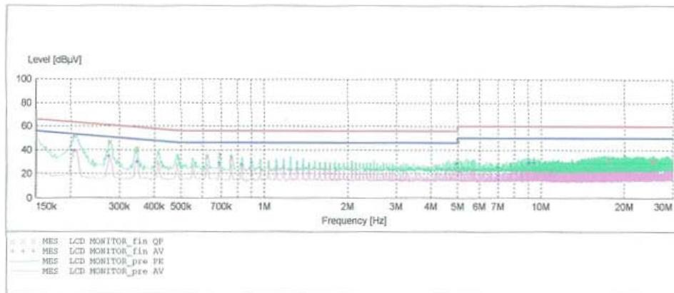
**MEASUREMENT RESULT: "LCD MONITOR\_fin QP"**
