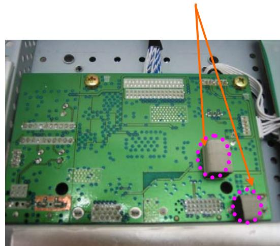
**3. Attach aluminum tape on the Rear frame.**
