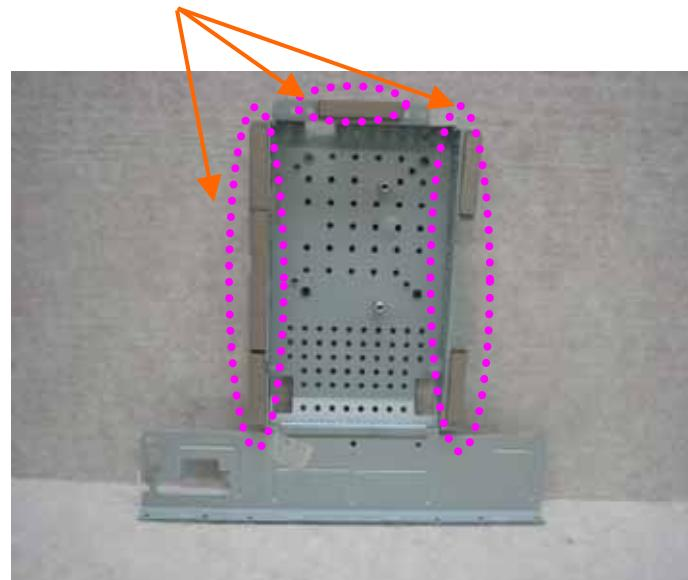
**2. Attach aluminum tape on the Rear frame.**
