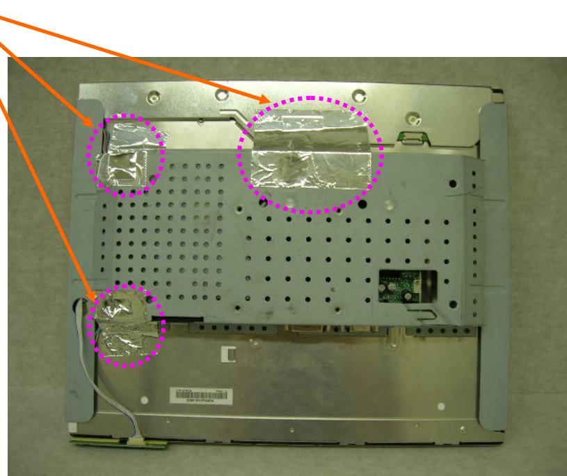
**2. Attach a gasket on the main frame to contact the lcd panel.**
