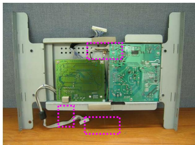
**2. Apply ferrite core to OSD signal line**
