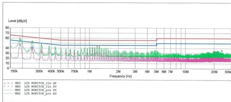
**MEASUREMENT RESULT: "LCD MONITOR\_fin QP"**
