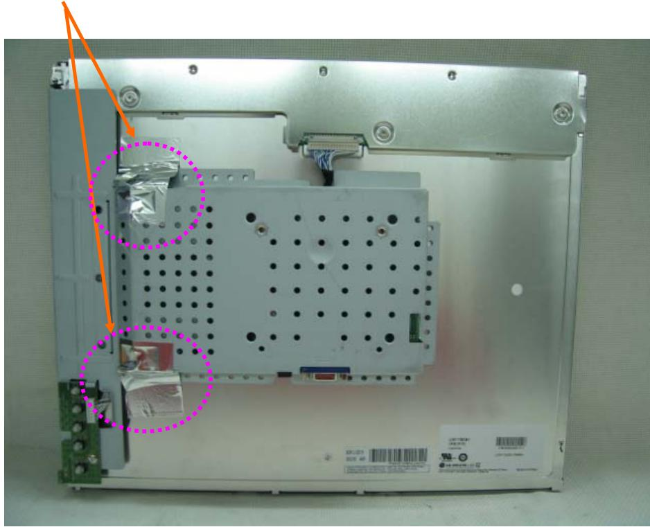
**2. Attach a gasket on the main frame to contact the lcd panel**
