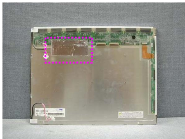
**4. Apply a ferrite Core to the OSD board signal cable**
