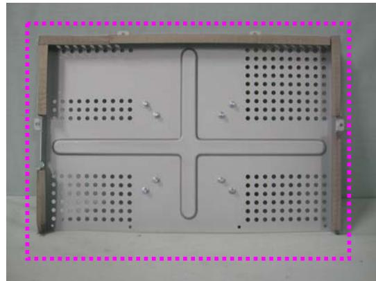
**2. Attach a gasket between Main Frame and LCD panel**
