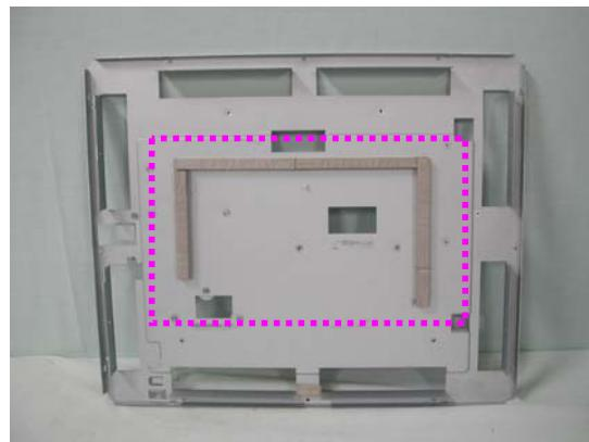
**3. Attach a gasket on the LCD panel**
