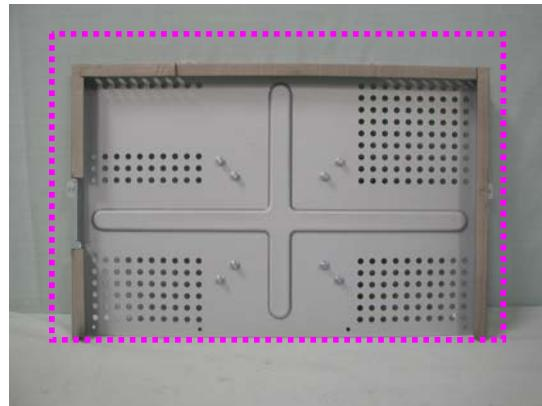
**2. Attach a gasket between Main Frame and LCD panel**
