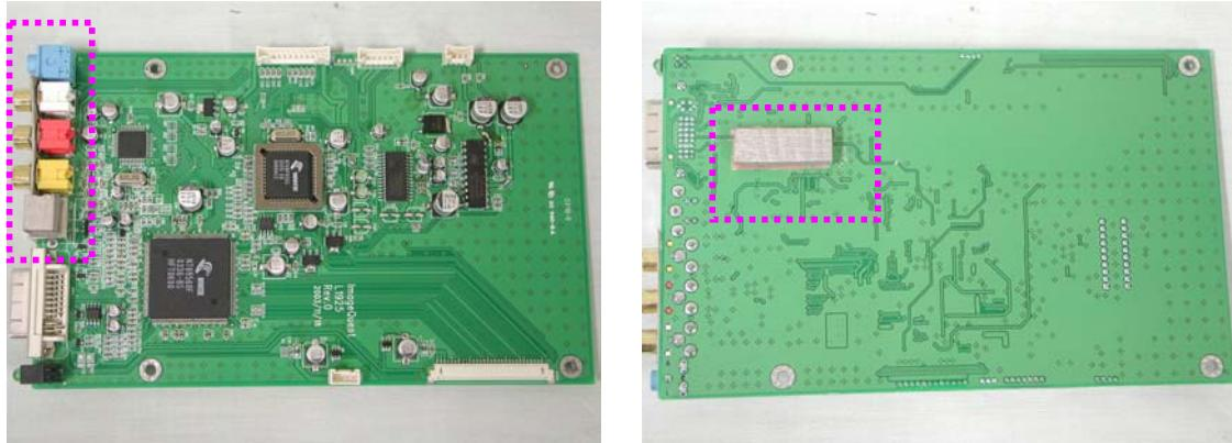
3. Attach a gasket on the LCD panel
