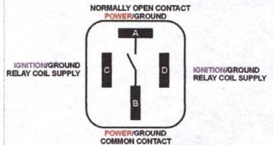
**ALL PINS.** – each pin of the NOSTART relay is used to pickup power or ground when either is applied. This process is automatic, hence no polarity considerations are necessary.
