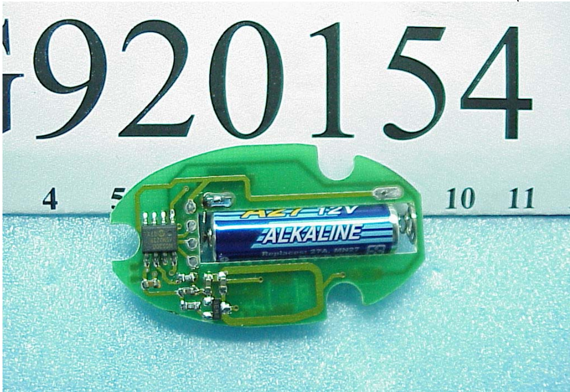
Photos 5 PCB View (Solder Side)
