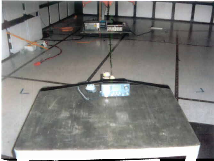
Set up photo for Radiated Emissions
