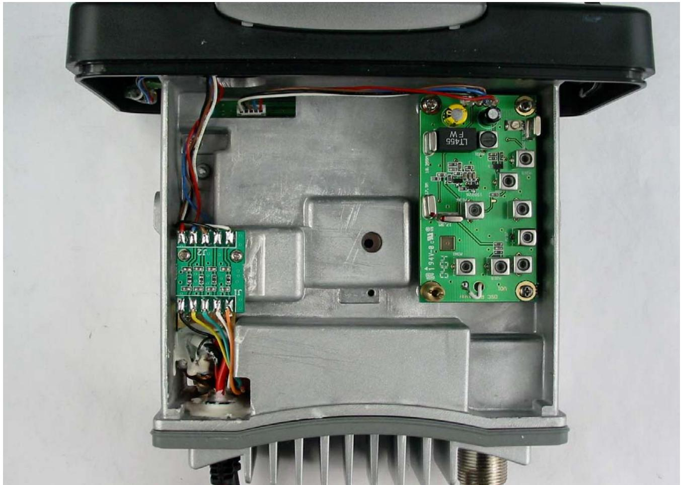
2nd top&gps filter top unit and assembly view
