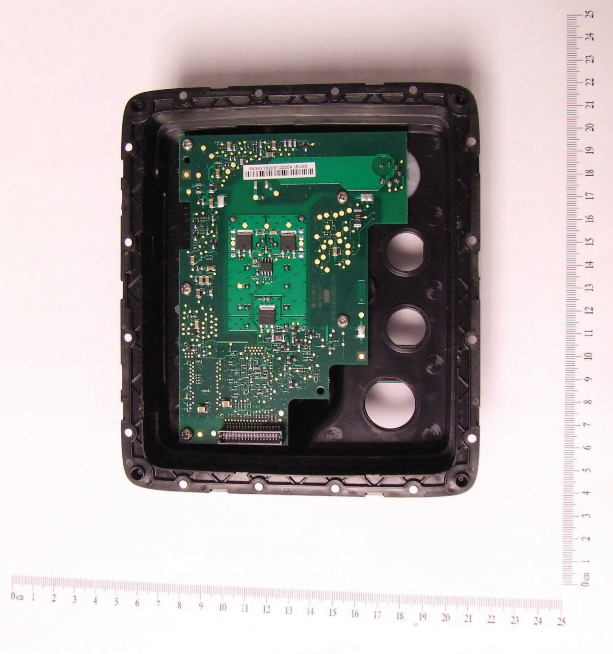
Figure 5 - Inside of A6 rear casing showing Sonar PCB (a67 only)
