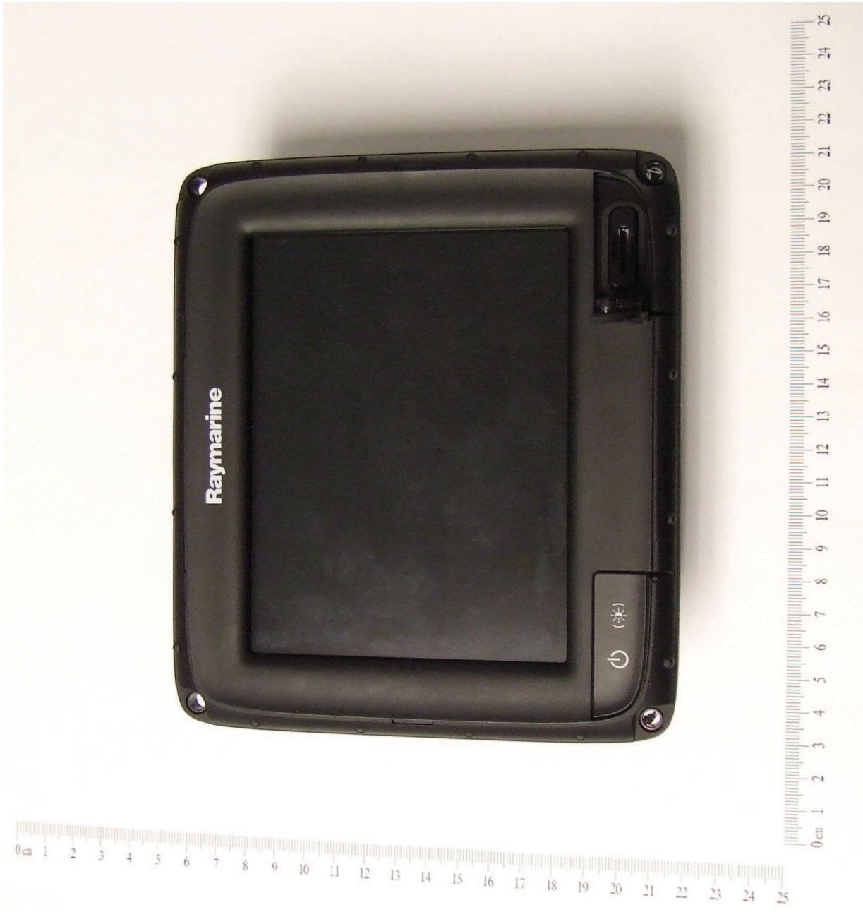
Figure 1 - Bezel removed & Micro SD Reader door open
