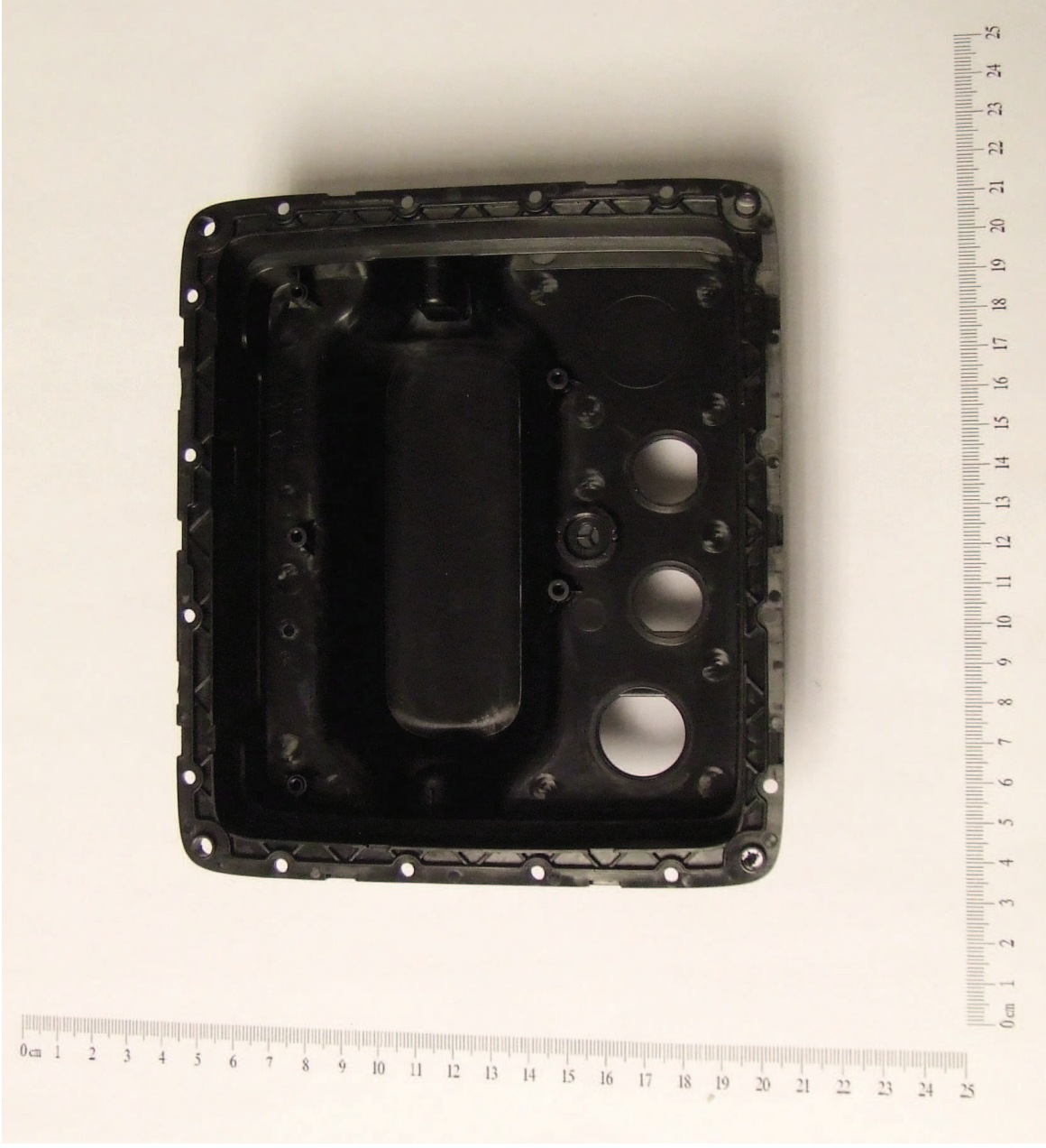
Figure 3 - Inside rear of a65 (no Sonar connector)
