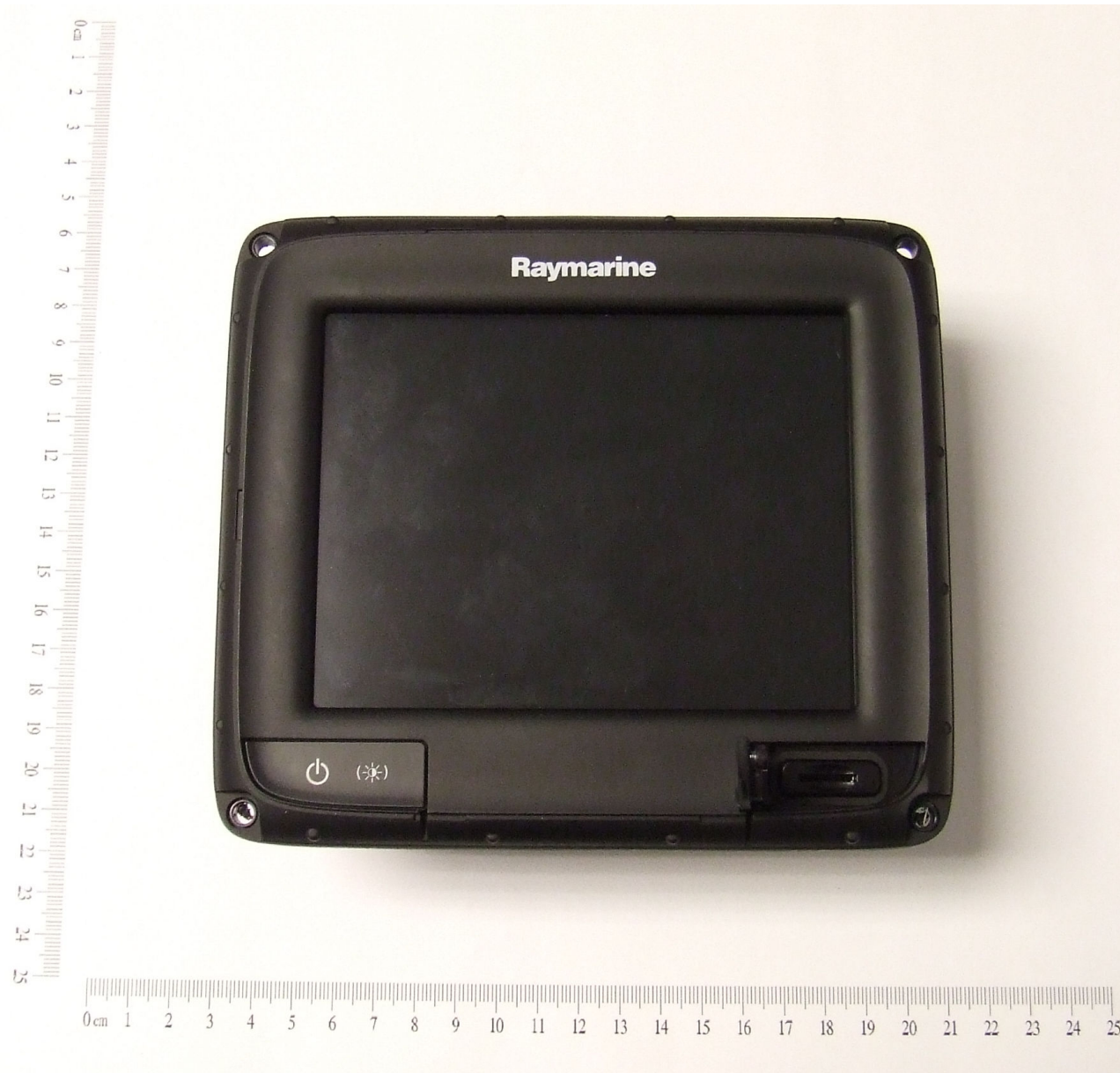
Figure 1 - Bezel removed & Micro SD Reader door open
