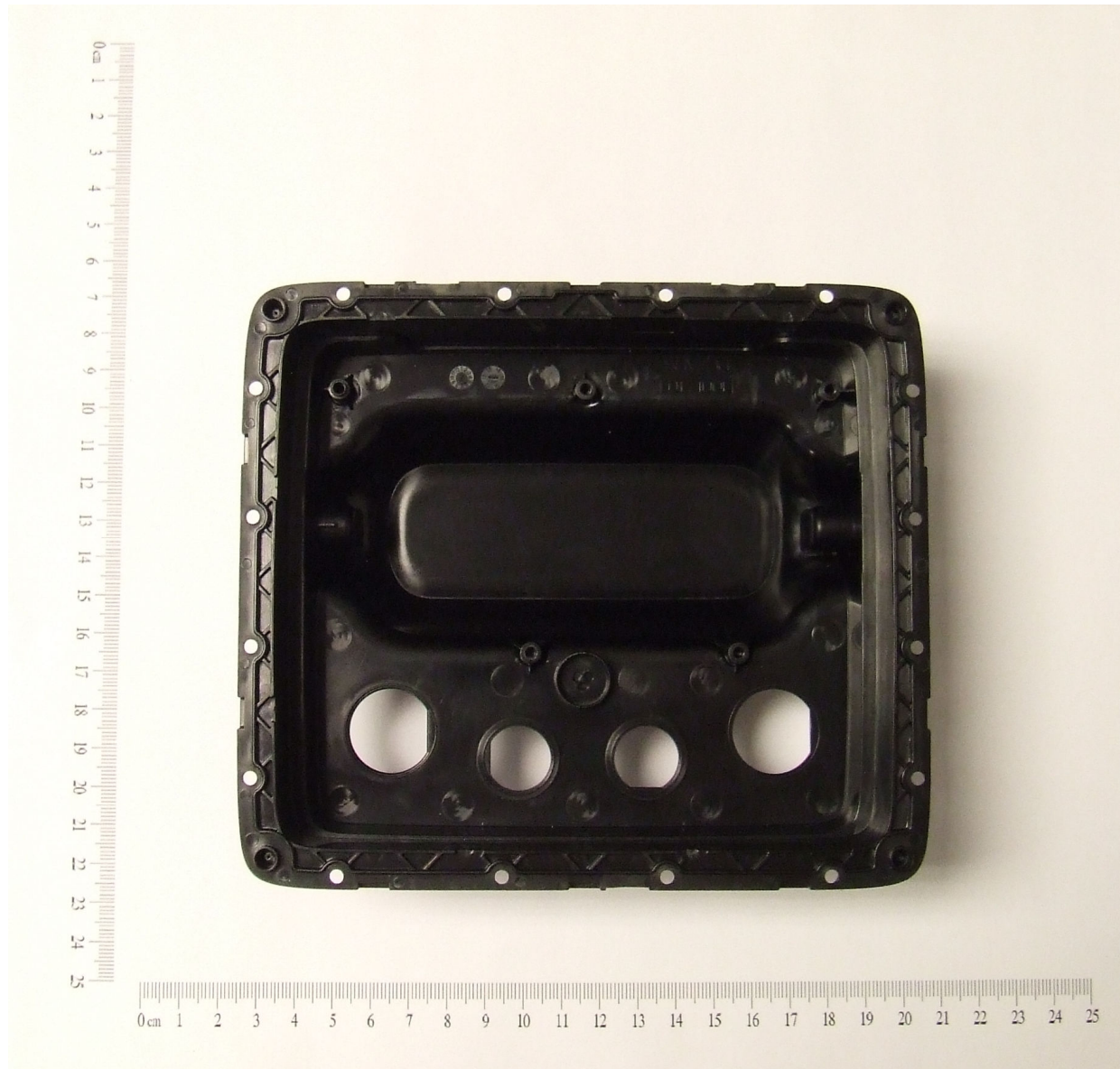
Figure 4 - Inside rear of a67 (for Sonar connector)
