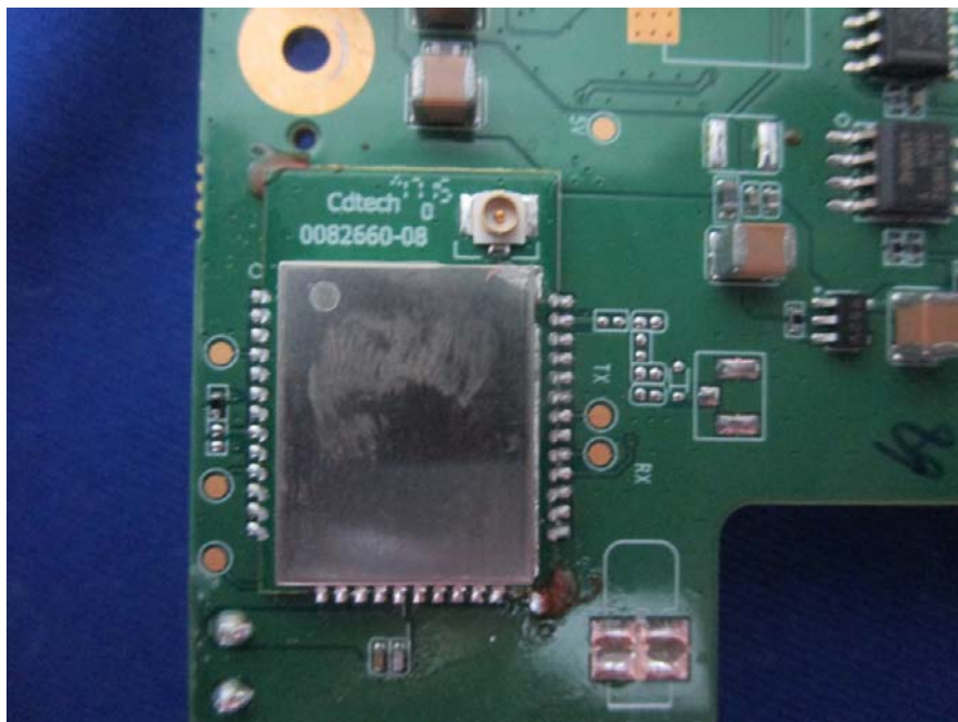
EUT – RF Module View
