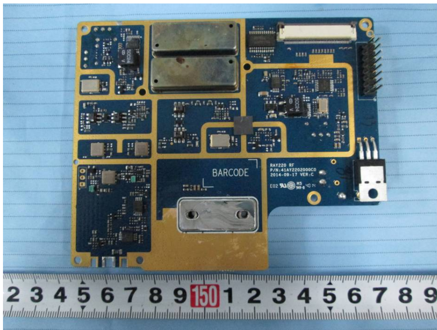
EUT –Base Main Board 1 Bottom View 1
