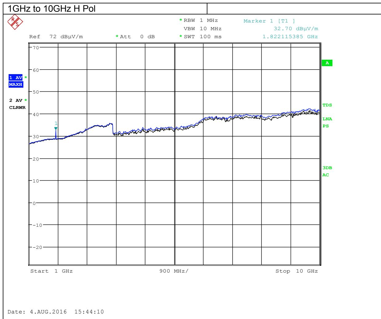
**Comments:** Unit 003 ran in constant talker for 1GHz to 10GHz range, and with a 2% duty cycle for the 916MHz range to give correct quasi-peak level.
