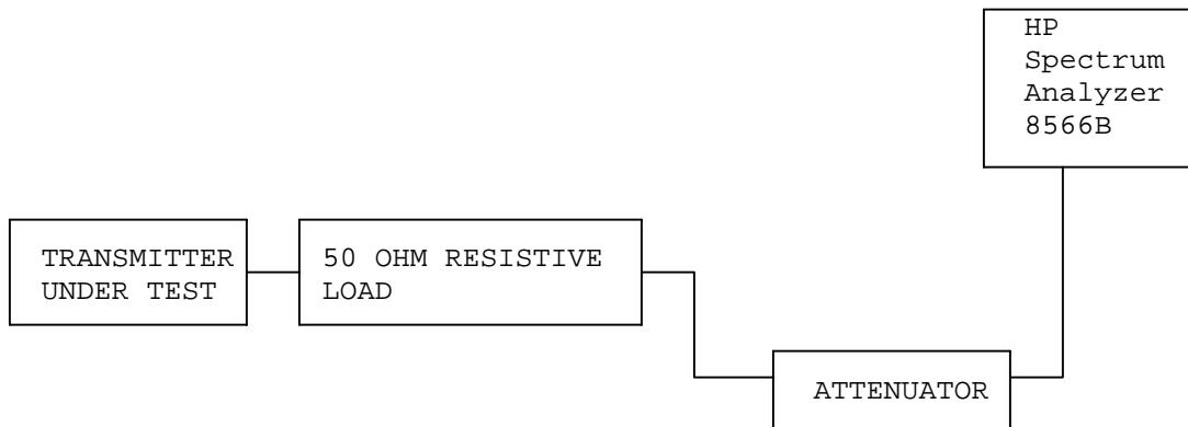
NAME OF TEST: SPURIOUS EMISSIONS AT ANTENNA TERMINALS
