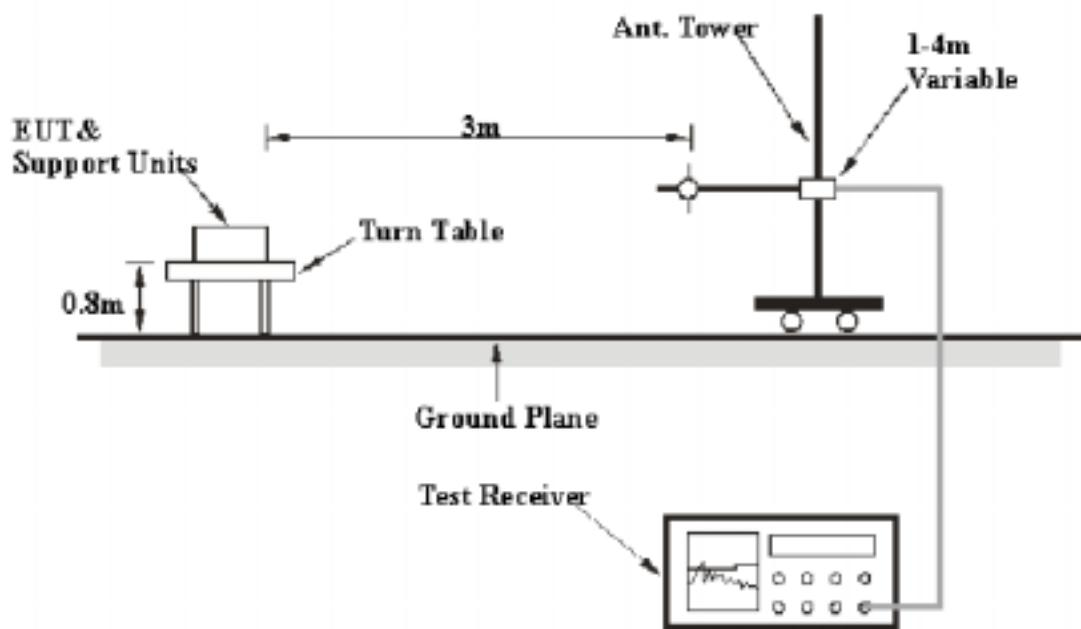
The radiated emission tests were performed in the 3 meters chamber B test site, using the setup accordance with the ANSI C63.4-2003. The specification used was the FCC Part 15 Class B limits.
