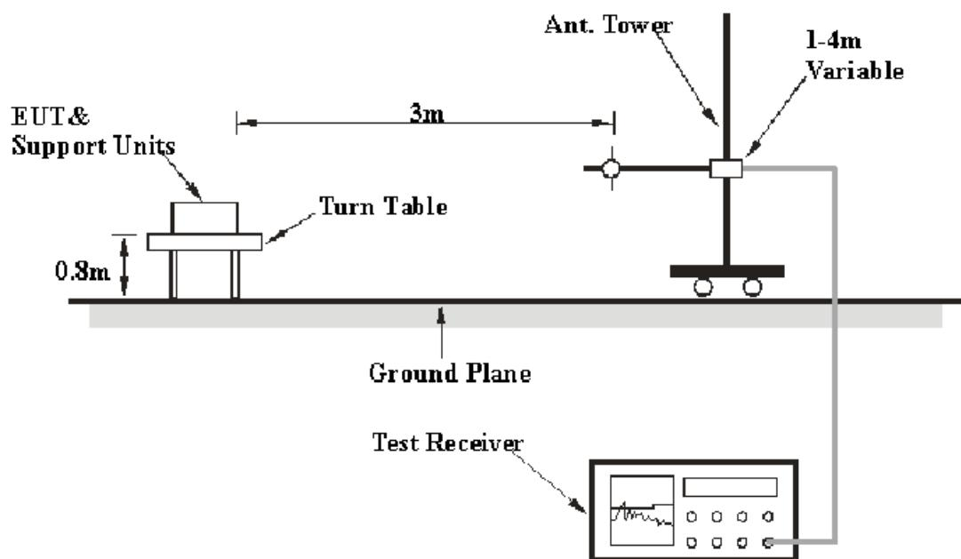
The radiated emission tests were performed in the chamber A test site, using the setup accordance with the ANSI C63.4-2003. The specification used was the FCC 15.109 limits.
