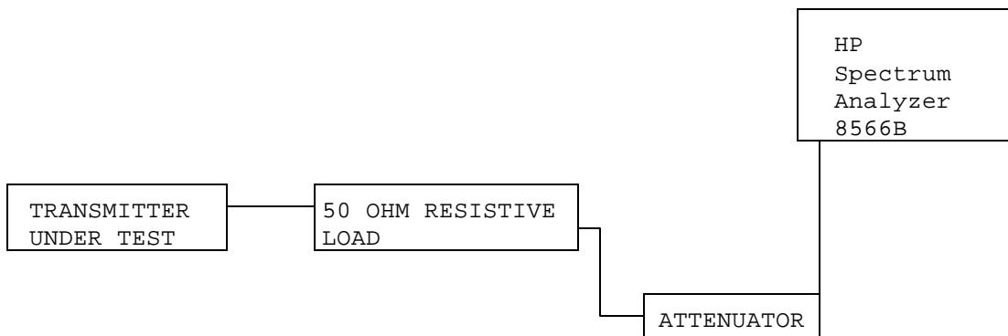
NAME OF TEST: SPURIOUS EMISSIONS AT ANTENNA TERMINALS
