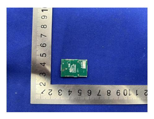
Integrated sample (Because the module just a highly integrated RF transceiver. It doesn't have integrated MCU or CPU. So didn't have ability to process data .It must be used in conjunction with MCU or controller accomplish sending and receiving functions.)
