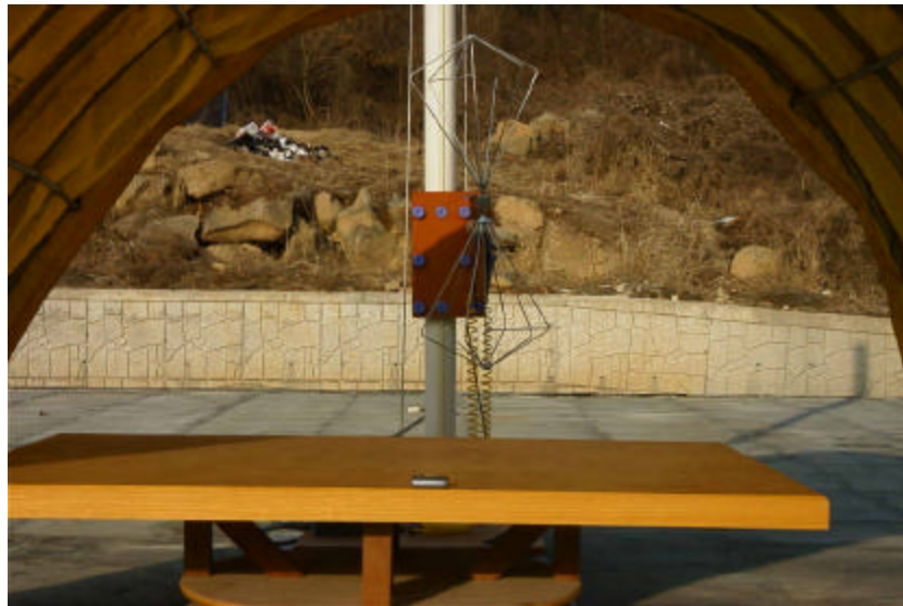
Photograph 1 : Setup for radiated Emissions
