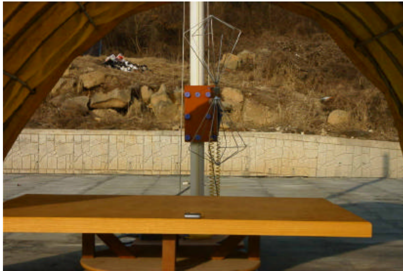
Photograph 1 : Setup for radiated Emissions
