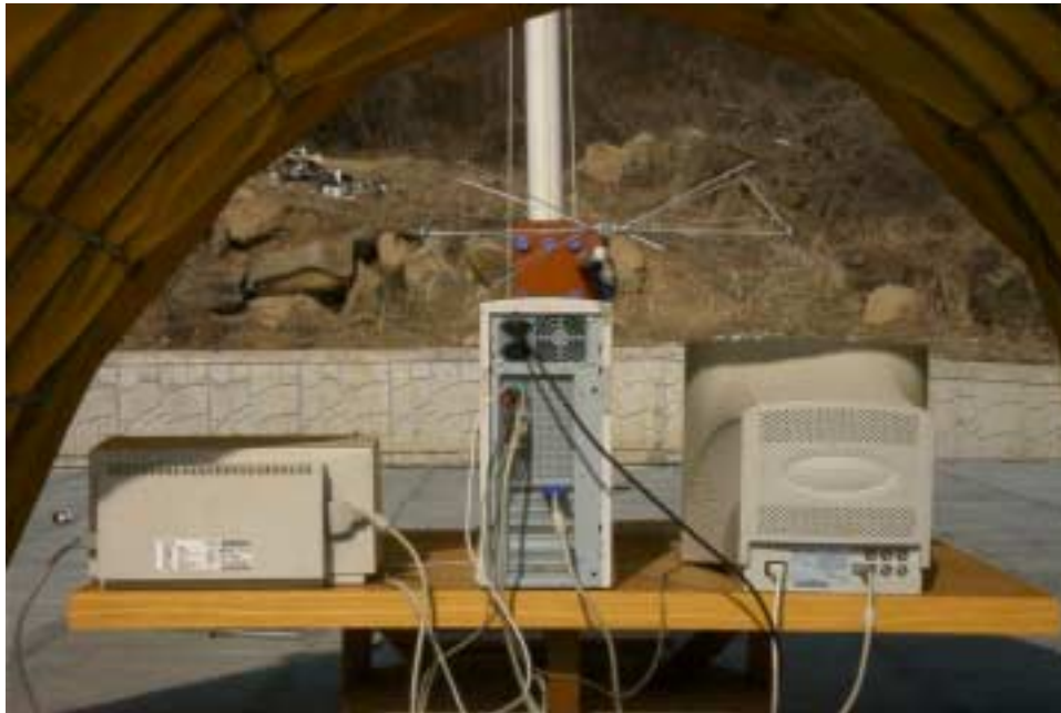
Photograph 1 : Setup for radiated Emissions
