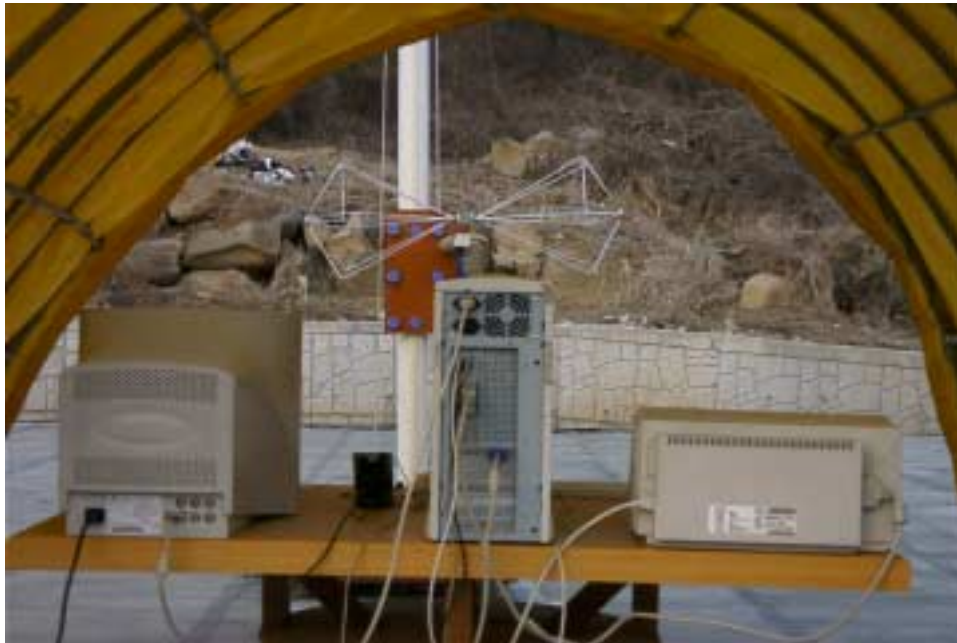
Photograph 1 : Setup for radiated Emissions
