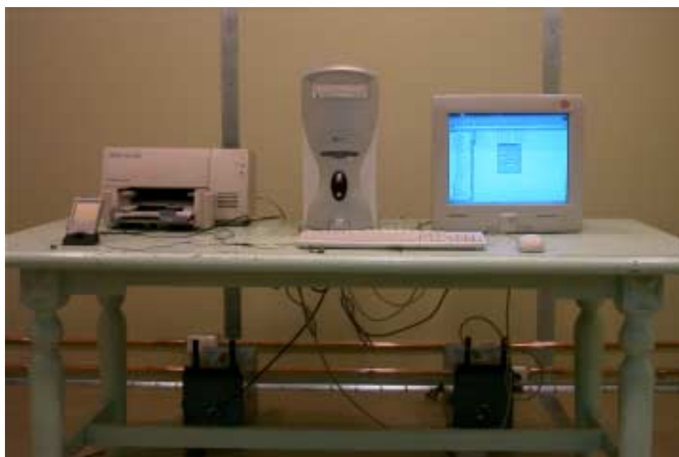
Photograph 2 : Setup for Conducted Emissions
