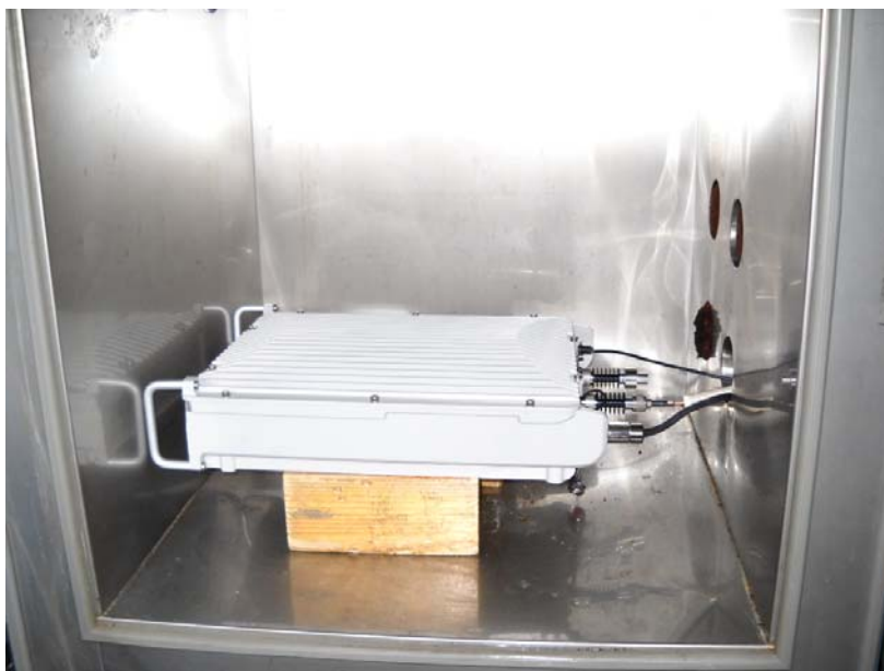
Photograph No.8 Frequency stability measurement setup
