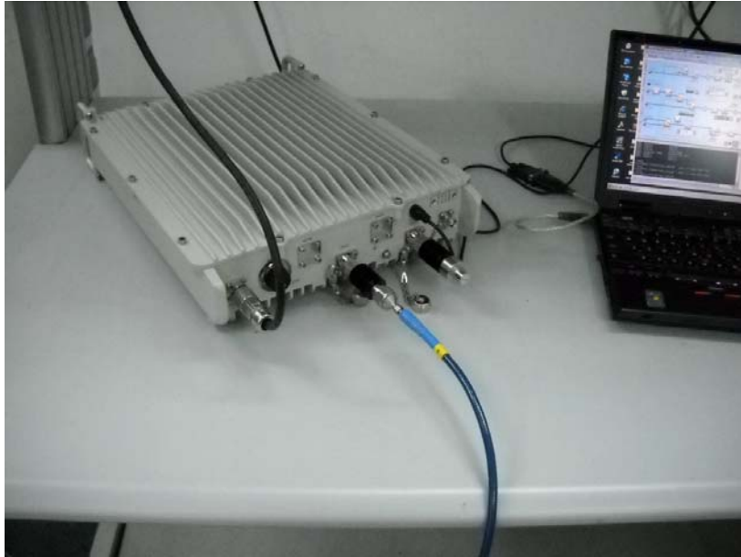
Photograph No.3 Conducted spurious emissions measurement setup
