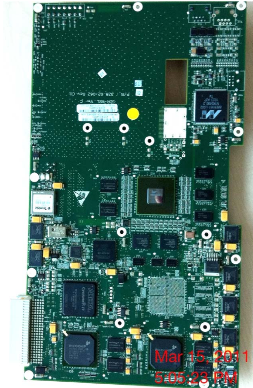
Photograph No.6 “uMAXe/AirGrid 3.65 GHz” digital PCB rear side view
