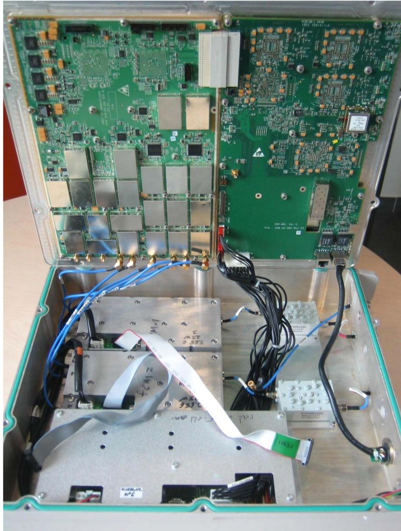
Photograph No.1 “uMAXe/AirGrid 3.65 GHz” internal view
