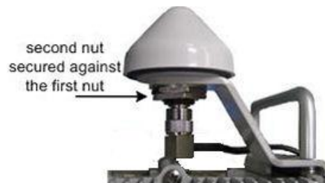
Figure 16 - GPS antenna assembled on bracket
