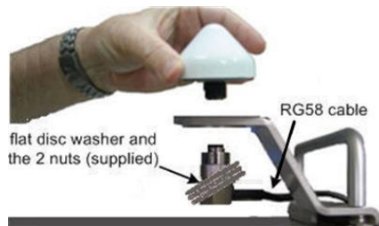
Figure 15 - Attach GPS antenna to RG58 cable
