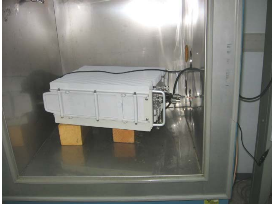
Photograph No.9 Frequency stability measurement setup
