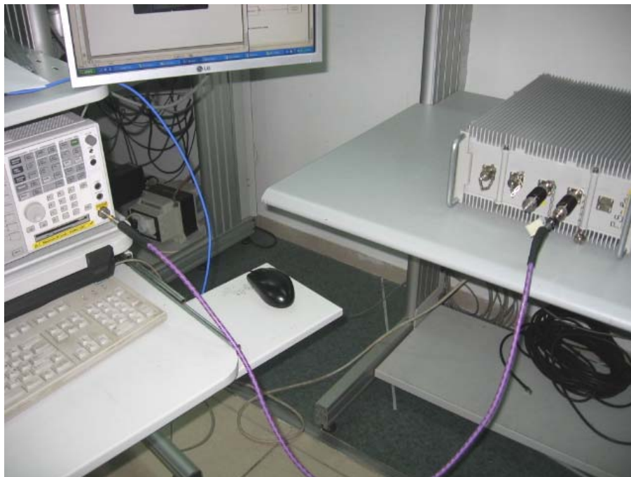
Photograph No.1 Peak output power and occupied bandwidth measurement setup
