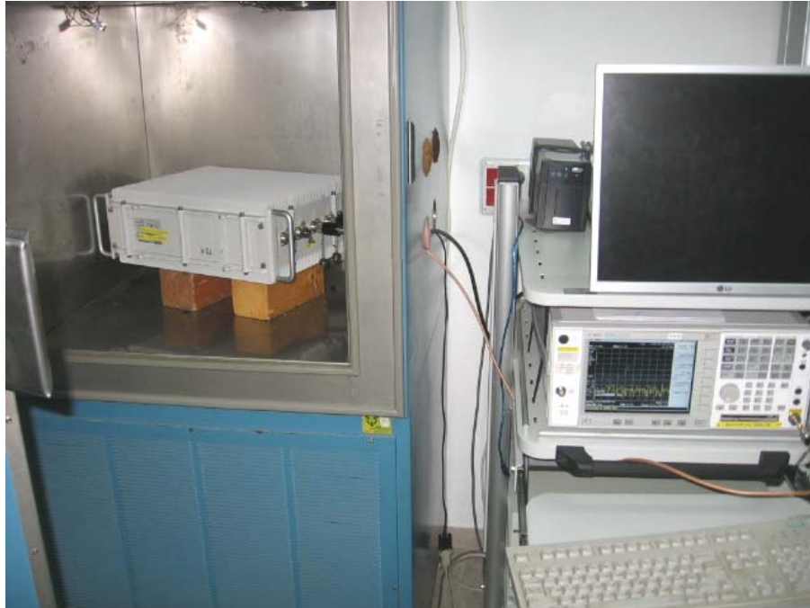
Photograph No.9 Frequency stability measurement setup
