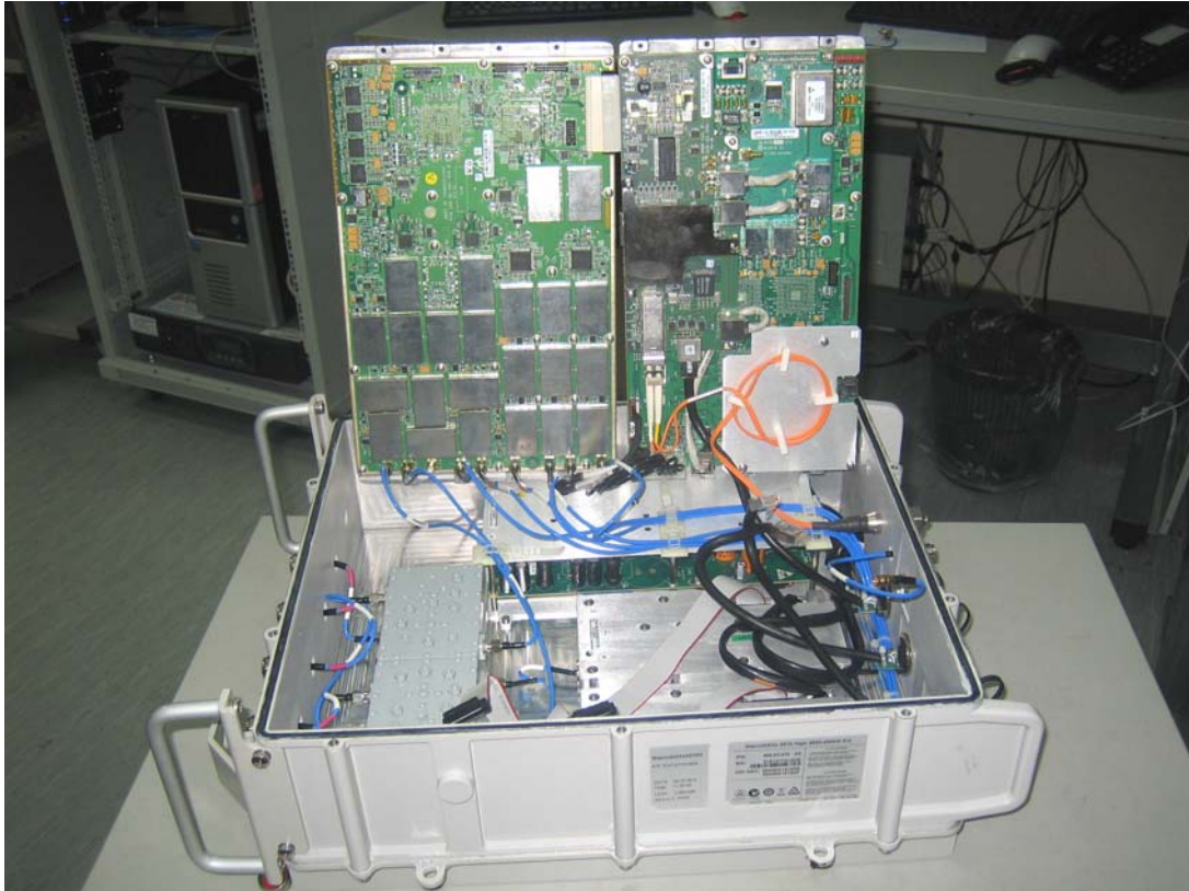
Photograph No.1 “MacroMAXe 2510 Mid” internal view
