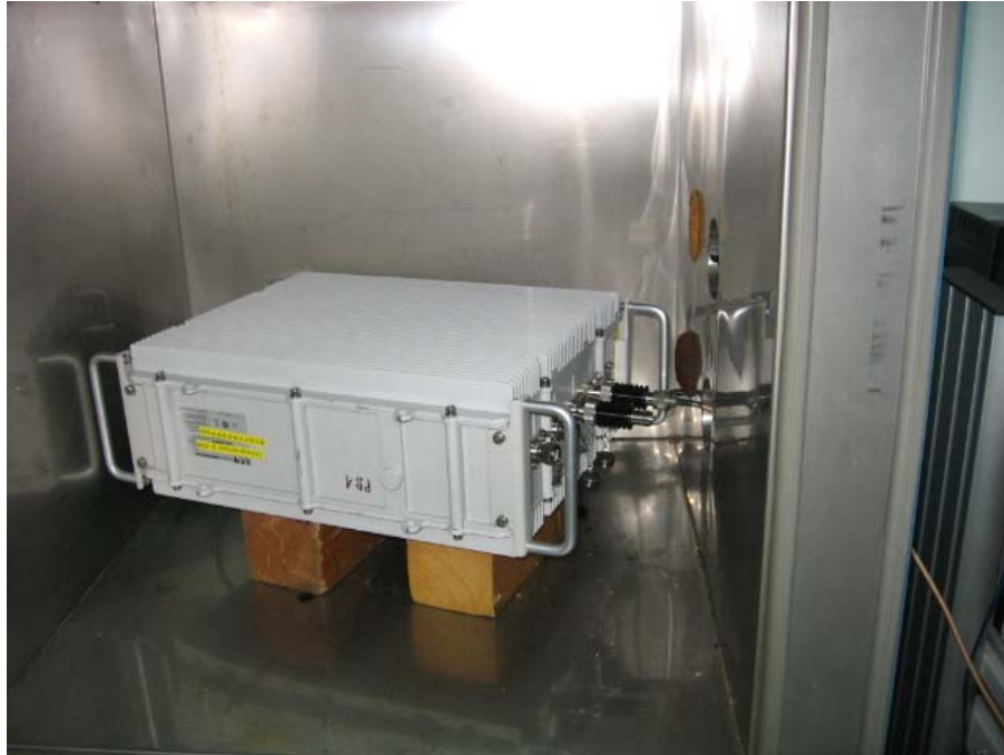
Photograph No.8 Frequency stability measurement setup
