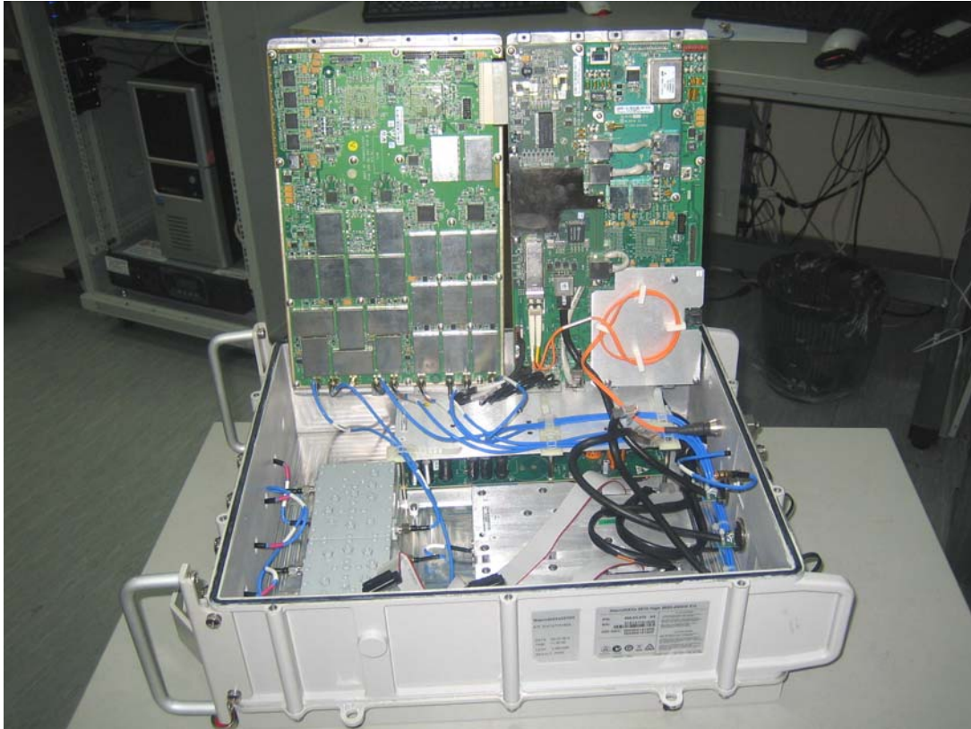
Photograph No.1 “MacroMAXe 2510L” internal view
