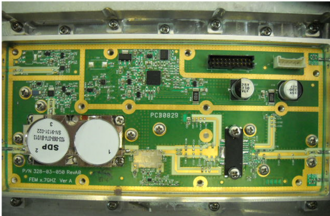
Photograph No.8 RF power amplifier internal view
