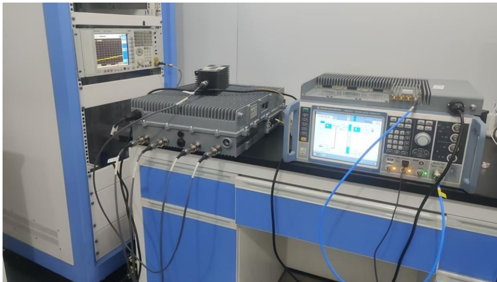
RF conducted test setup
