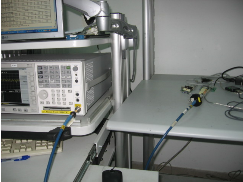
Photograph No.2 Conducted spurious measurement setup
