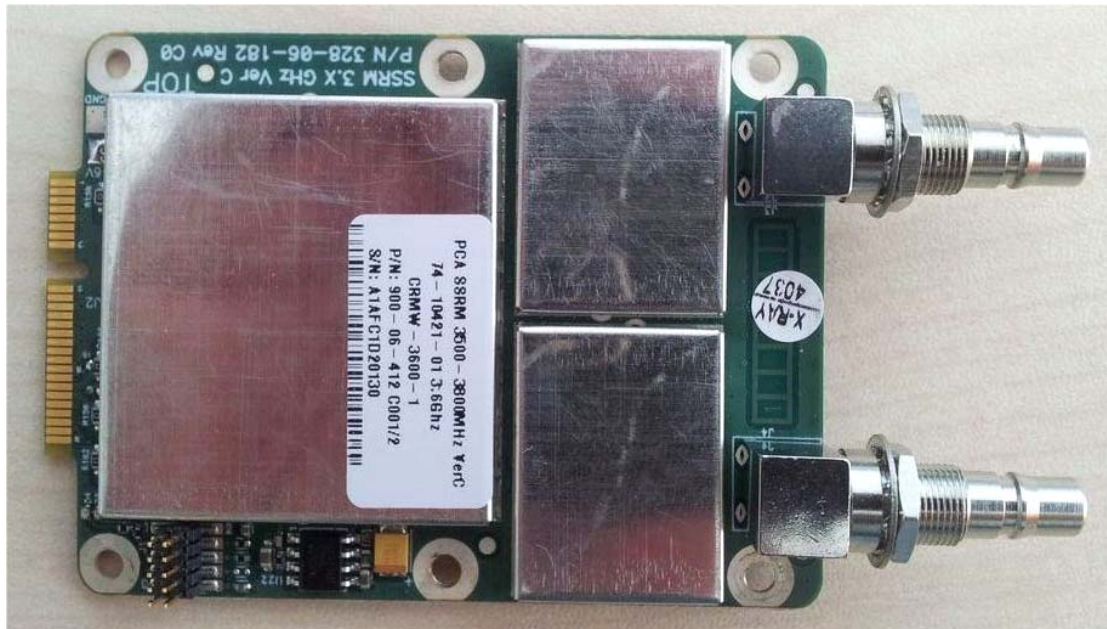
Photograph No.1 SSRM 3.65GHz module top view
