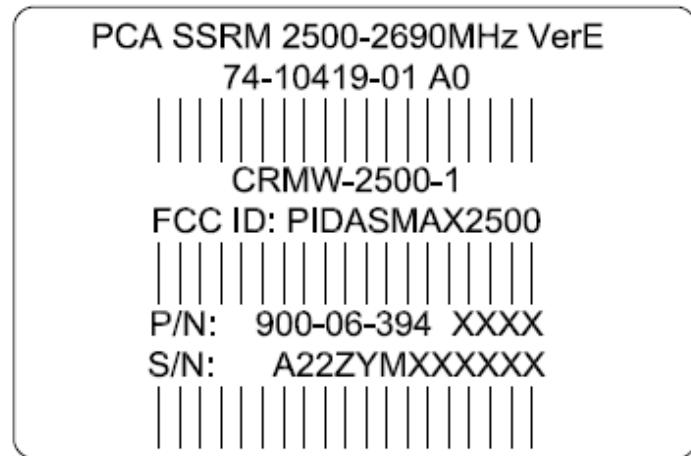
**SSRM 2.5 GHz module, label with FCC ID:PIDASMAX2500 location**
