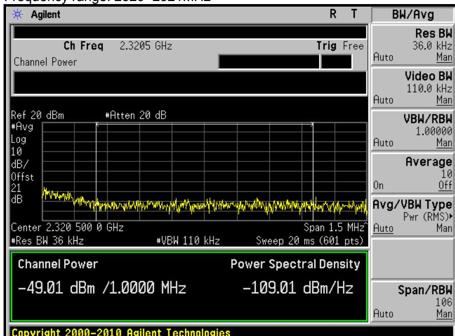
**NOTE:** Due to instrument noise floor limitation, the full investigating range is subdivided into 3 to 4 plots
