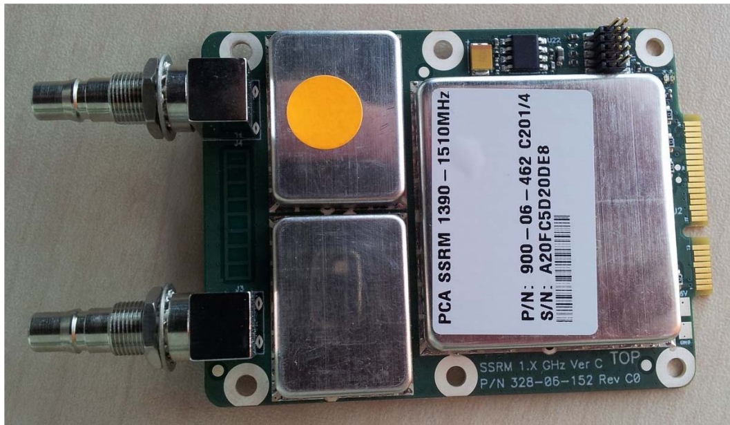
Photograph No.1 SSRM 1.4 GHz module top view
