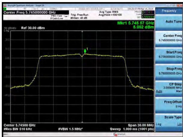
U-NII-3, 802.11ac VHT20, Channel No.: 157
