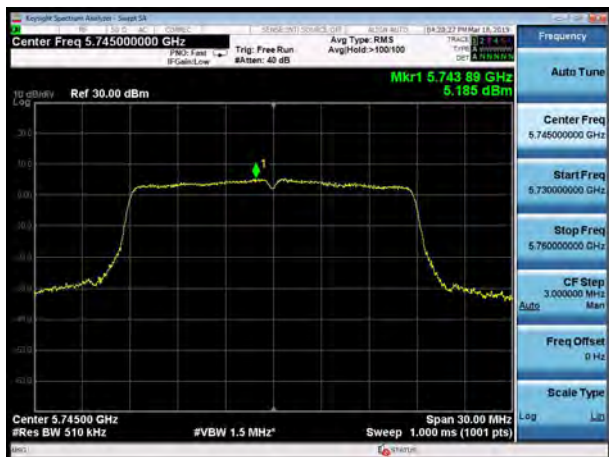
U-NII-3, 802.11ac VHT20, Channel No.: 157
