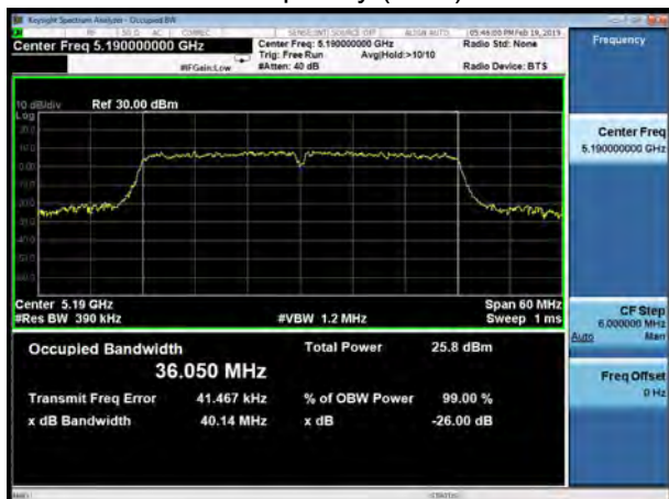
U-NII-1, 802.11n HT40 Carrier frequency (MHz): 5230
