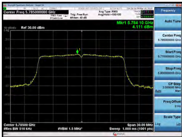
U-NII-3, 802.11ac VHT20, Channel No.: 165
