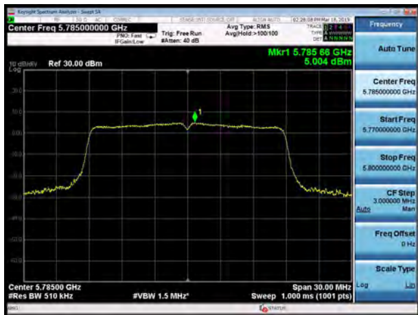
U-NII-3, 802.11ac VHT20, Channel No.: 165
