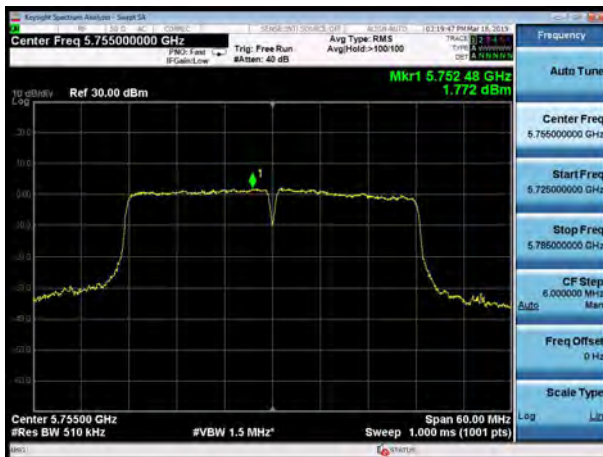
U-NII-3, 802.11ac VHT40, Channel No.: 151
