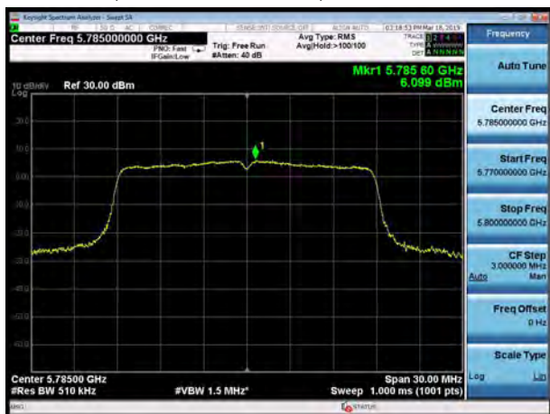
U-NII-3, 802.11ac VHT20, Channel No.: 165
