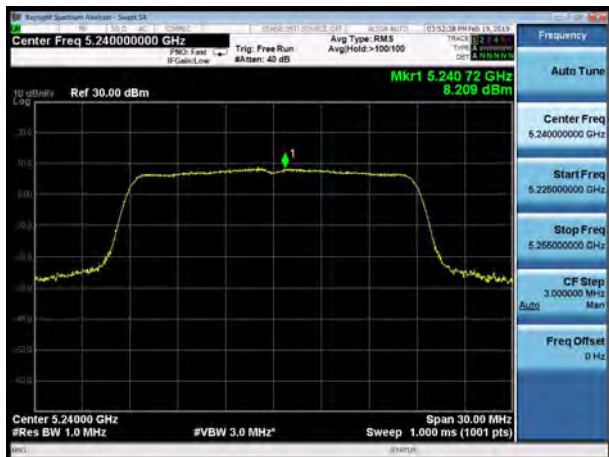
U-NII-1, 802.11ac VHT20, Channel No.: 48
