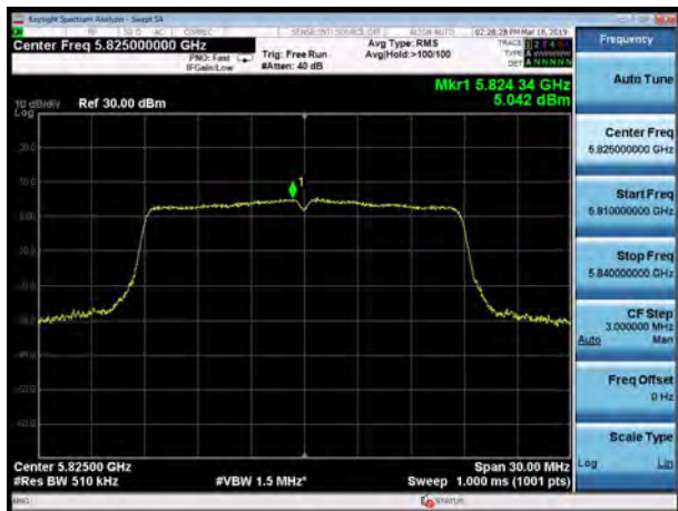
U-NII-3, 802.11ac VHT20, Channel No.: 165
