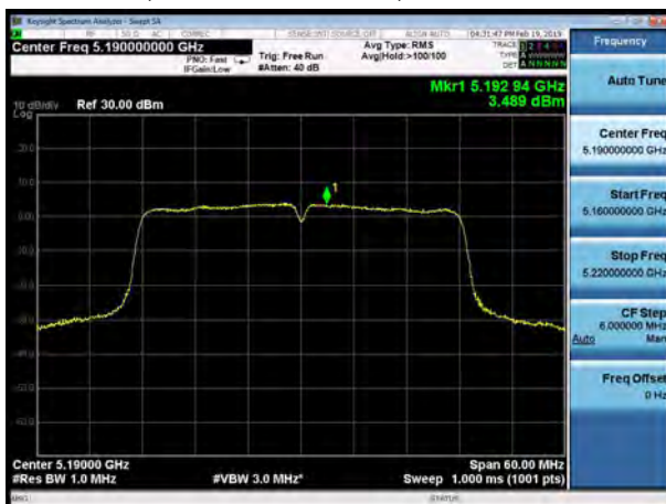
U-NII-1, 802.11ac VHT40, Channel No.: 38
