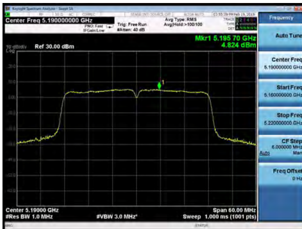
U-NII-1, 802.11ac VHT40, Channel No.: 38
