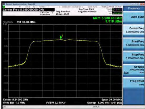
U-NII-1, 802.11ac VHT20, Channel No.: 48
