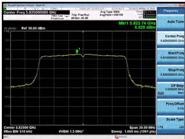
U-NII-3, 802.11ac VHT20, Channel No.: 165
