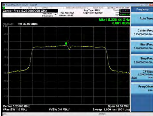
U-NII-1, 802.11ac VHT40, Channel No.: 38
