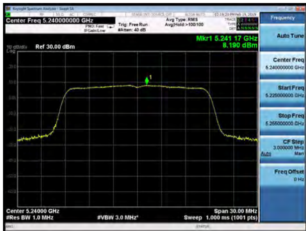
U-NII-1, 802.11ac VHT20, Channel No.: 48
