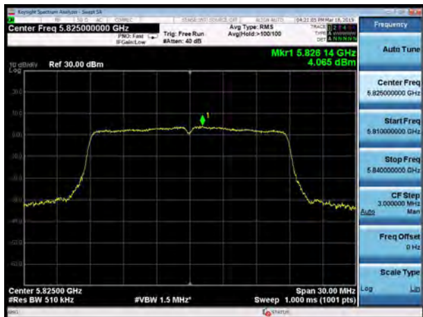
U-NII-3, 802.11ac VHT20, Channel No.: 165
