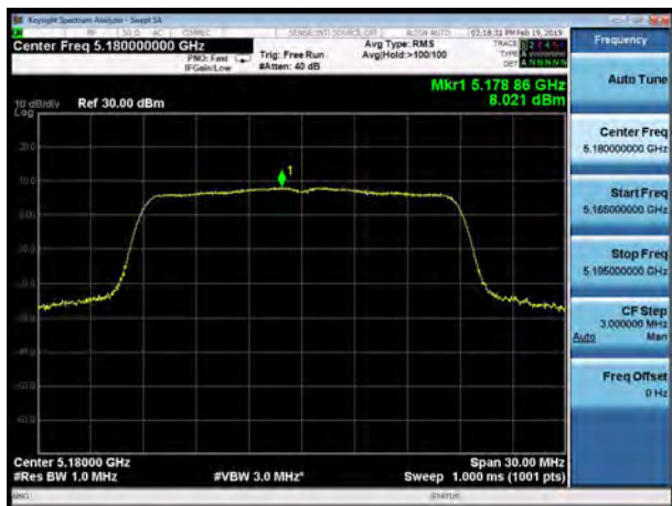
U-NII-1, 802.11ac VHT20, Channel No.: 40
