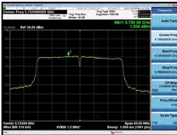
U-NII-3, 802.11ac VHT40, Channel No.: 151
