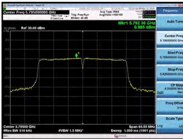
U-NII-3, 802.11ac VHT40, Channel No.: 151
