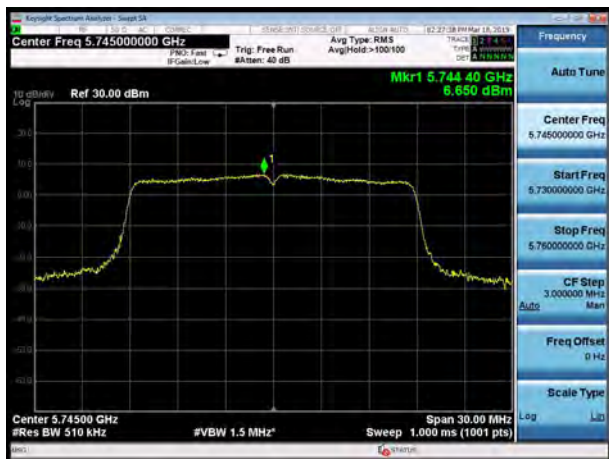
U-NII-3, 802.11ac VHT20, Channel No.: 157
