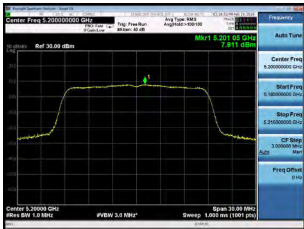
U-NII-1, 802.11ac VHT20, Channel No.: 48
