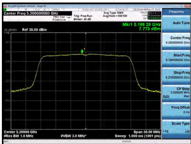
U-NII-1, 802.11ac VHT20, Channel No.: 48
