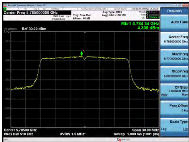
U-NII-3, 802.11ac VHT20, Channel No.: 165
