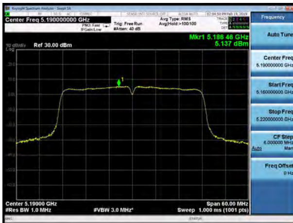
U-NII-1, 802.11ac VHT40, Channel No.: 38
