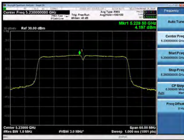
U-NII-1, 802.11ac VHT40, Channel No.: 38
