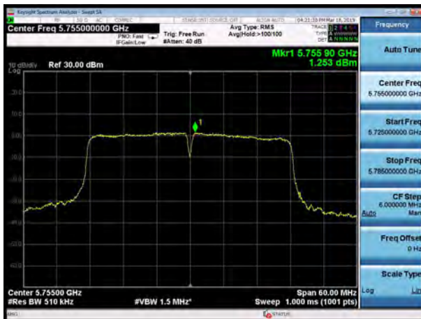
U-NII-3, 802.11ac VHT40, Channel No.: 151
