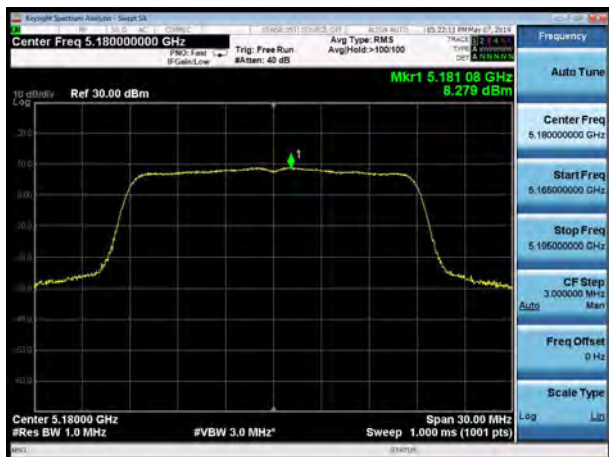
U-NII-1, 802.11ac VHT20, Channel No.: 40
