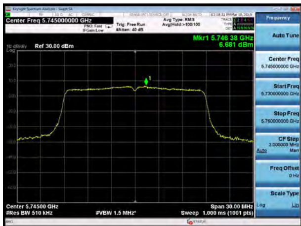
U-NII-3, 802.11ac VHT20, Channel No.: 157
