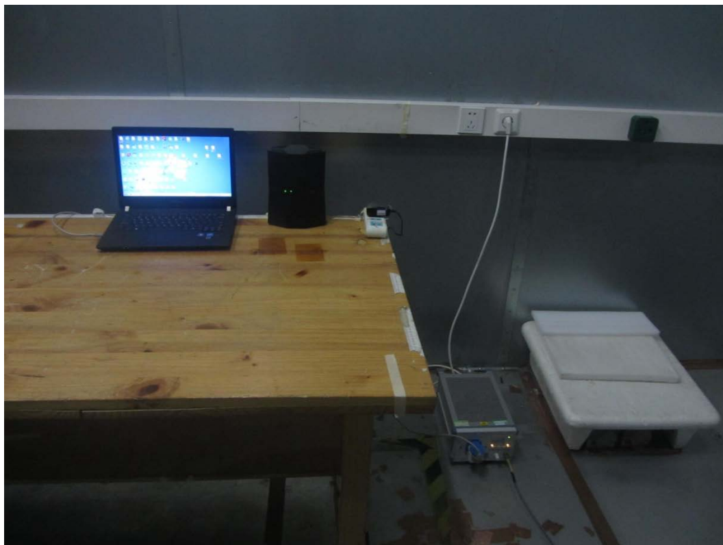
Picture 3 Conducted Emission Test Setup
