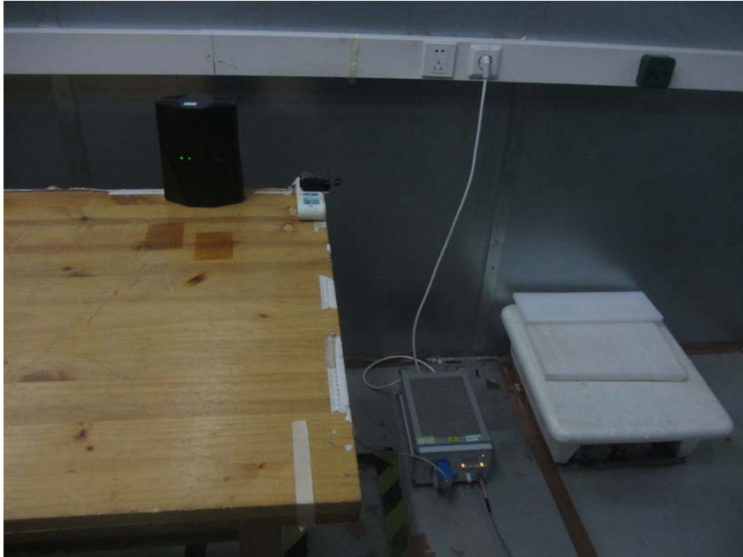
Picture 3 Conducted Emission Test Setup
