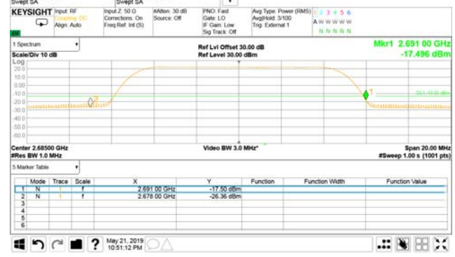
Plot 7.3.4 Spurious emission at band edges test results at low carrier frequency
