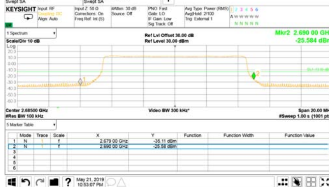
Plot 7.3.4 Spurious emission at band edges test results at low carrier frequency
